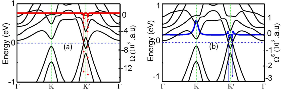
**Figure S3.** (a) and (b) Band structures (black solid curves) for the SbH sheet with one Mo atom deposited on  $\text{Sb}_A$  atom in the  $1 \times 1$  unit cell with a 3% tensile strain. The red dots in (a) and blue dots in (b) denote the Berry curvatures and spin Berry curvatures for the whole valence bands, respectively.
