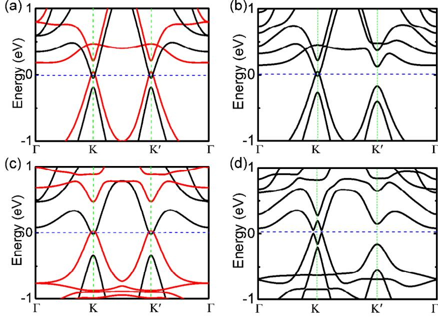
**Figure S1.** (a) and (b) Band structures for the  $1 \times 1$  unit cell of Cr@SbH with a 5% tensile strain applied, without and with SOC considered, respectively. The red and black curves denote the spin-up and spin-down states, respectively. (c) and (d) are the same as (a) and (b) except for W@SbH.
