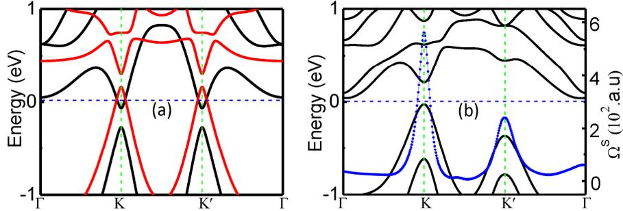
**Figure S2.** (a) and (b) Band structures for the  $1 \times 1$  unit cell of Mo@BiH without and with SOC, respectively. The red and black curves in (a) denote the spin-up and spin-down states, respectively. The blue dots in (b) denote the spin Berry curvatures for the whole valence bands. Chern number and spin Chern number of the system are 0 and  $\sim 1$ , respectively.
